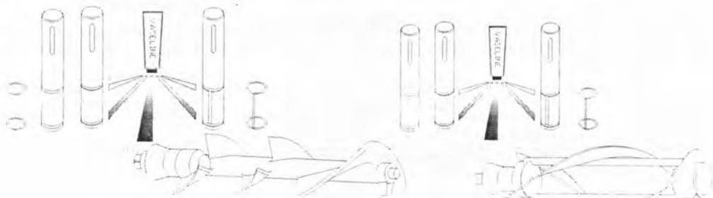
**Notice:** Before installing the piston, O-ring for piston, beater and gasket for beater, you should lubricate vaseline (lubricating vaseline onto the groove of the gasket, do not onto the beater's end ), using the vaseline frequently can extend the service life of components.
